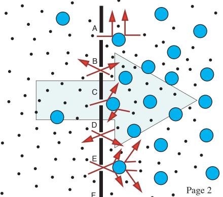
In the diagram at left, the higher solute concentration is clearly on the right side and the many "one-way valves" cause a net movement of water from the left to the right. Although there may be "one-way valves" on both sides of the semi-permeable membrane, the side with the greater concentration will see a greater movement of water to that side.
